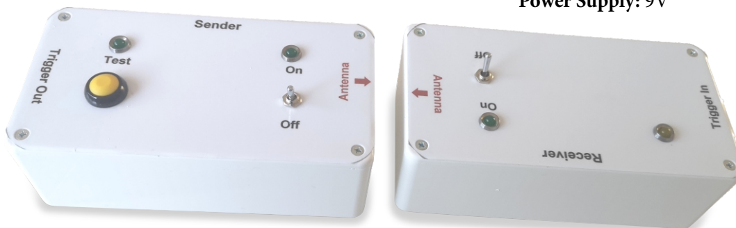
Wireless trigger unit WTU1 with sender and receiver unit
