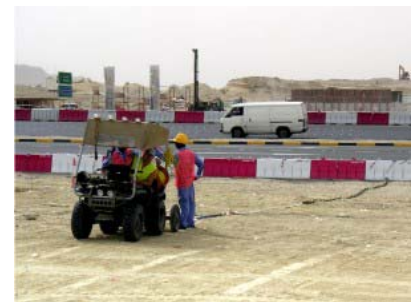
System for land survey of large areas. Note the geophone string (landstreamer) behind the quad bike.
