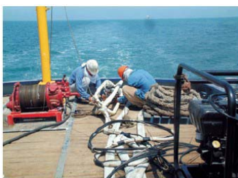
MASW-equipment (air gun and hydrophone string)
